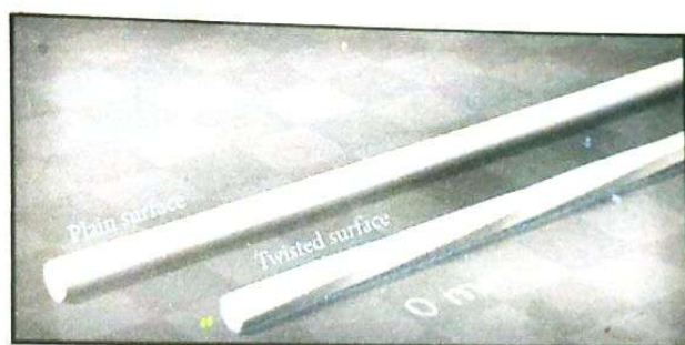
FIGURE 9: Simple 3D models of two types of geometrical surfaces printed to verify how the surface design can modify the photocatalytic experiments.
